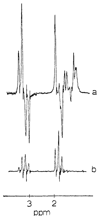
Figure 1. Reaction of ethyllithium with ethyl iodide in benzene. (a) Spectrum taken during the reaction, showing the methylene ( \delta 3.2) and methyl protons ( \delta 1.85) of ethyl iodide and butane ( \delta 1.0-1.6) (3.5-2.5-ppm region scanned with a spectrum amplitude twice that of the remainder of spectrum). (b) Reference spectrum of ethyl iodide.
